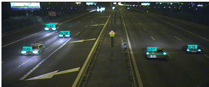
Figure 6: Result of night mode vehicle detection
