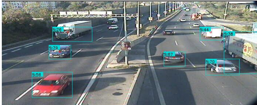
Figure 5: Result of daylight mode vehicle detection
